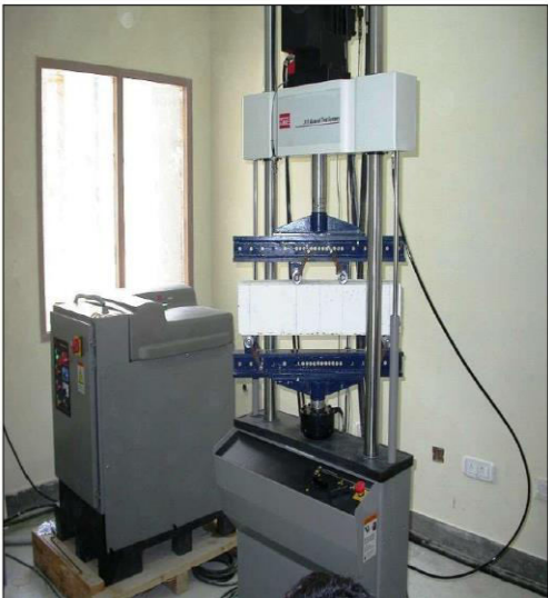
CUBE COMPRESION TEST
