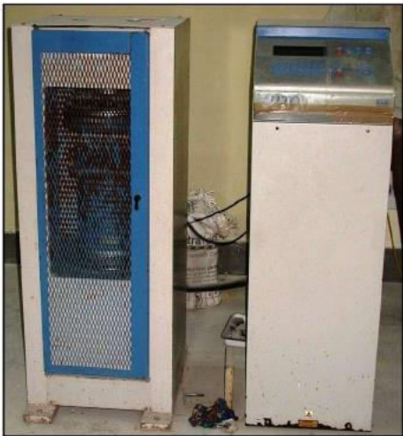
CUBE COMPRESION TEST
