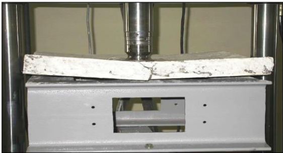
Figure 5.18 Panel failure in static load
