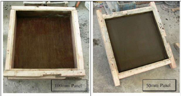
Figure 4.7 Wooden moulds for panels
